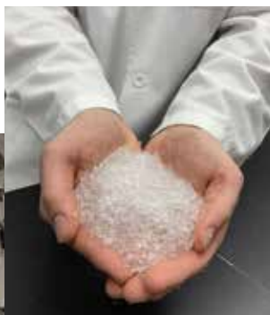
◀◀ Figure 2. Ecovia has developed a method to produce biopolymer products that mimic the structure and absorbency properties of conventional synthetic superabsorbent materials. These super-absorbents can be placed into diapers and other personal care products to make them completely biodegradable.
